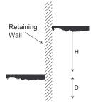
Maximum height of wall (H) and the corresponding minimum driven depth (D) depend on the type of soil and the strength of the sheet piling. Where the fill differs from the soil into which the piling is driven, use the H & D values of the respective soil type.
