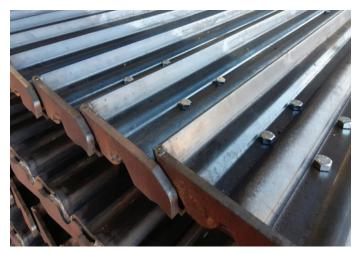
This unique technology ensures that Australian Rollforming Manufacturers Carrier Slats are precision made to exacting tolerances, particularly in terms of the radii of the leading and trailing edges and the pitch of the chain.
