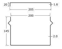
Steel base thicknesses are usually 1.2, 1.6, 2.0, and 3.0mm, but other thicknesses, materials and profile dimensions can also be provided. All Australian Rollforming Manufacturers Cable Trunking is available with Z275, Z450 and Z600 zinc coatings.
