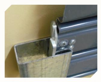
Rollformed from 3.00mm thick pre-galvanised steel and available in any length, Windlock has the added benefit of eliminating the costly and time consuming on-site fabrication of the channel (which includes cutting, welding and painting), and in turn also eliminates the inherent OH&S issues associated with on-site fabrication.
