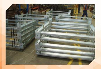
5 kilometres of conveyor sections were rollformed from hi-tensile galvanised steel coil in Australian Rollforming's factory in Dandenong, Victoria.
